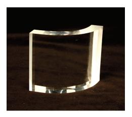
Eljen light guides are fabricated from cast acrylic materials. Cast acrylic is a clear and colorless plastic which generally has good optical clarity and good mechanical properties. It has very little natural scintillation response to ionizing radiation.
